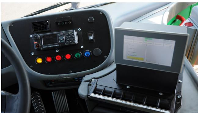
State-of-the-art on-board computers provide drivers with information and manage the entire vehicle periphery in all vehicles.
